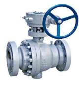
Trunnion ball valve 20 Product type Construction Top entry 4" to 36" Size range CL 150, CL 300, CL 600, CL 900, CL Pressure rating range 1500, CL 2500 Carbon steel, Low carbon steel, SS, Material range **Duplex SS** Stem, Ball: SS, Duplex SS, Seat : Internals PTFE Ends Flanged, BWE Lever operator, Gear Operator operator, Electrical Actuator
