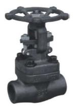
15 Product type Globe Valve OS & Y, Bolted or Welded Bonnet Construction 1/2" to 2" Size range CL 800, CL 1500, Cl 2500 Pressure rating range Carbon steel, Low carbon steel, Material range Alloy steel, SS Disc, Seat: 13% Cr SS, SS, Stellite, Internals Stem: 13% Cr SS, SS Ends Flanged, BWE, SWE, Threaded Operator HW - Manual, Electrical Actuator
